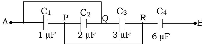
Calculate the equivalent capacitance between the points  $A$  and  $B$  in the following Figure :
